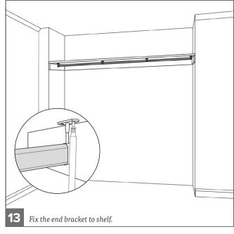
If your opening space is wider than 1.2m then we recommend fitting the vertical support as well.
