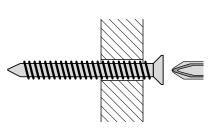
If you know you are fixing directly into a wooden batten, the screws provided do not require a plug.
