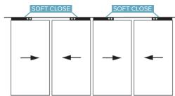
PLAN VIEW - Circles represent the amount of the soft close units as well as the positioning.
